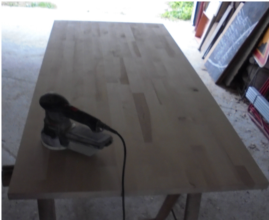
Figure 17: Tabletop being sanded.
