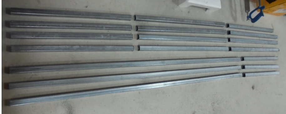
Figure 15: Steel tubes cut to length.
