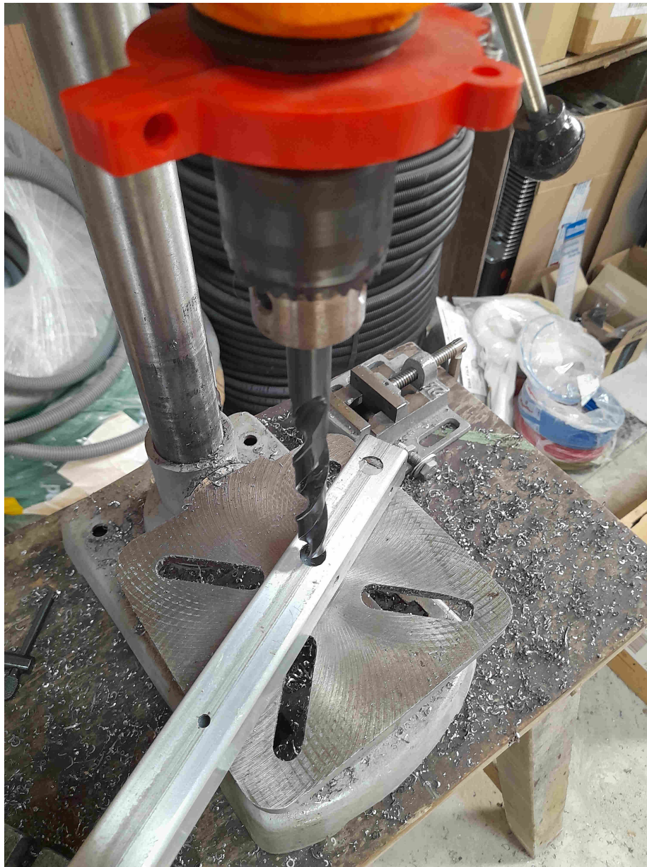
Figure 16: Drilling holes in the tubes.
