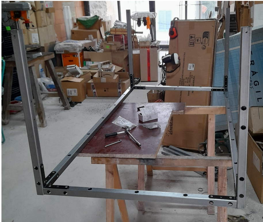
Figure 21: Assembled feet on the frame.
