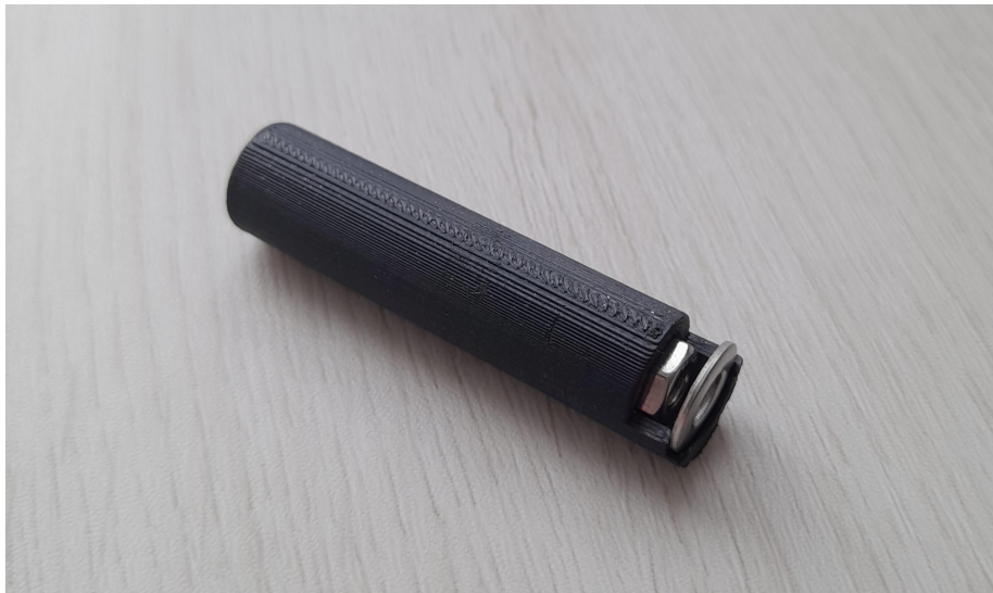
Figure 13: Fastener holder tool with nut and washer.
