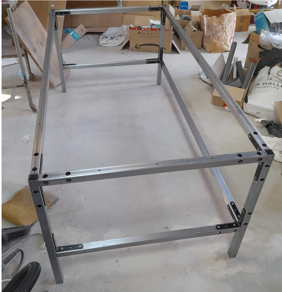
Figure 22: Assembled braces on the frame.
